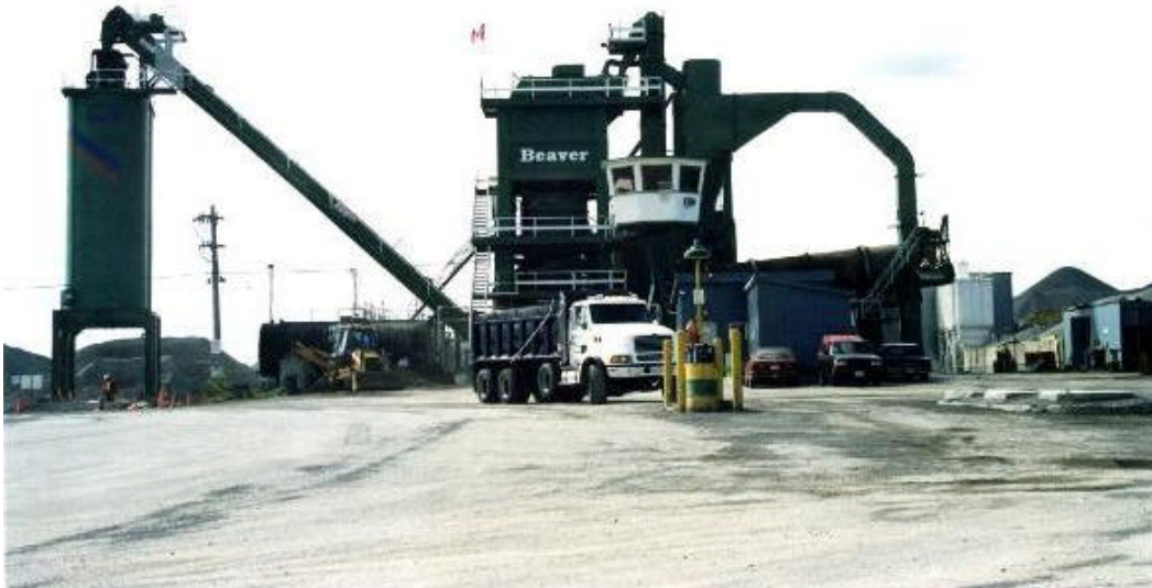
PHOTOGRAPH 2: Beaver Road Builders 8000 lb Barber Greene Batch Plant
