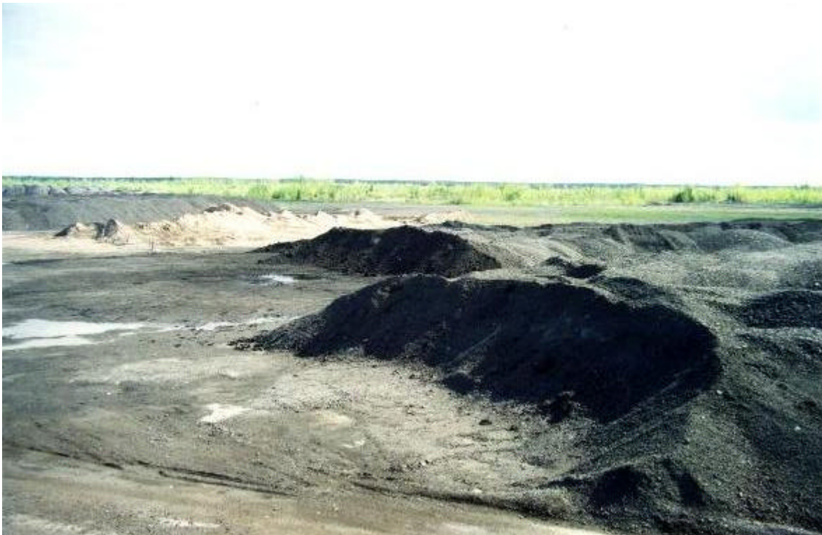
PHOTOGRAPH 1: Area Containing Various Stockpiles of Recycled Asphalt Pavement (RAP) Material from Different Construction Projects
